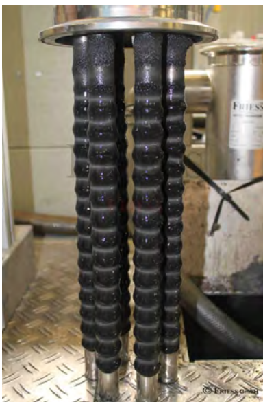
1) Contaminated magnetic bars 2) Operating principle magnetic filter rod
