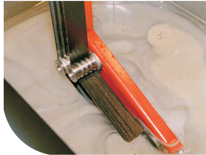
The skimmer belt draws the oil due to the movement it creates on the surface
