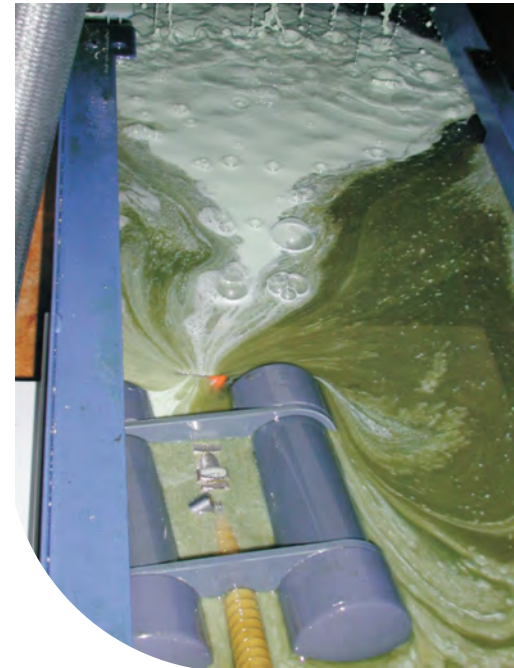
Suction float removes oil from emulsion
