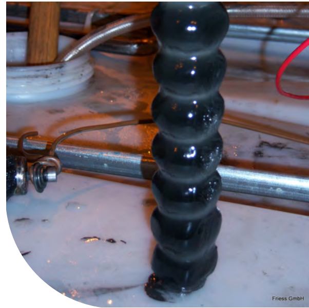
Dirt on magnetic filter rods
